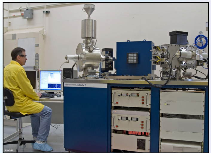
Mass spectrometry is used to determine the isotopic actinide ratios present in a sample. These ratios are useful for determining how a sample was processed and how old it is.
