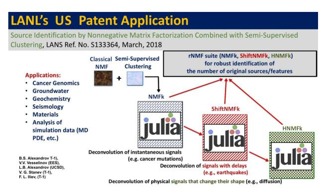
**rNMF Schematic**: A suit of three new methods and algorithms for data exploratory analysis, features extraction, data mining and dimension reduction based on subspace learning via robust Nonnegative Matrix Factorization (NMF) with a custom estimation of the unknown number of factors (features), and integrated Green's function, time delays, and other physical constraints.
