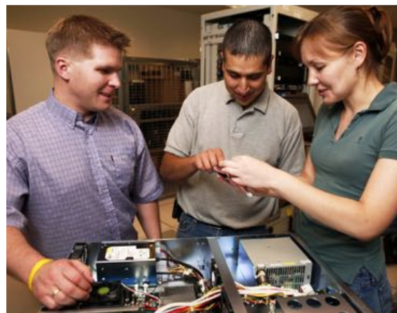
Instructor (left) and intern diagnosing compute node hardware
