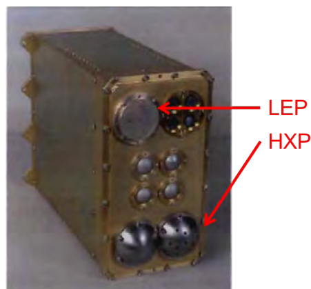
Figure 3: Energetic Particle Sensors on CXD. LEP: Low Energy Particle subsystem has 5 electron channels. HXP: High-energy X-ray and Particle subsystem has 7 electron channels. Eleven electron channels on 19 block IIR and IIF satellites.
